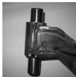
Figure 11. Kingpin After Cleaning
