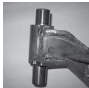
Figure 22. Kingpin After Cleaning
