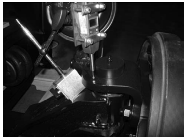
Figure 6 Vertical End Play Checking
