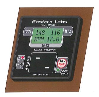
Cut a 2-3/8" square hole in dash. Take counter apart and reassemble with the face in front of the dash and the rest (aluminum ring, back plate, terminal block, & junction box cover) from behind the dash.
