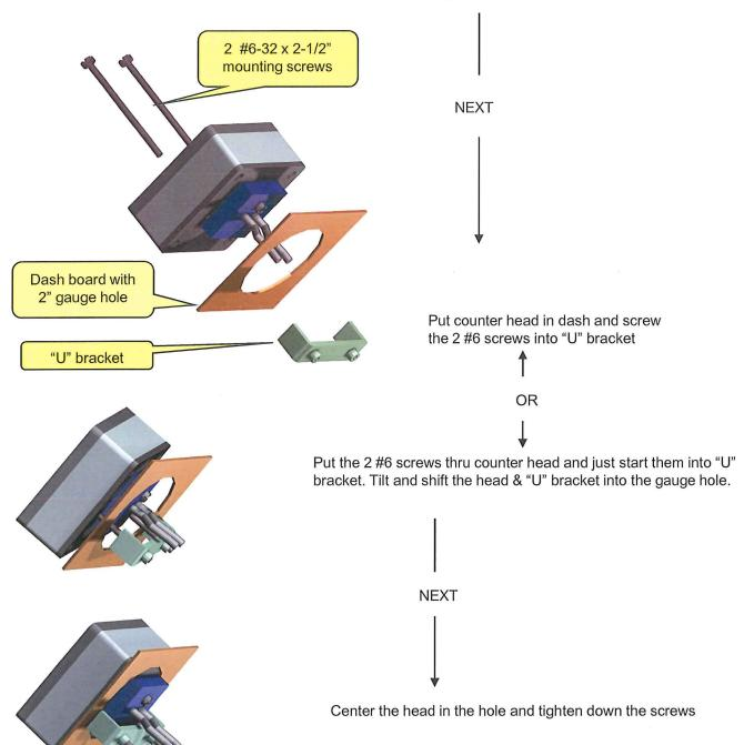
To remove the head in the future just remove 1 #6 screw completely and loosen the other. This will allow you room to tilt and shift the head & "U" bracket out.
