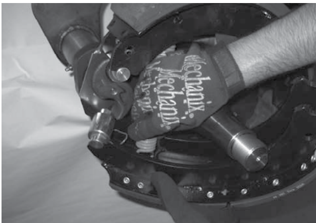
Figure 47. Removal of Return Spring
