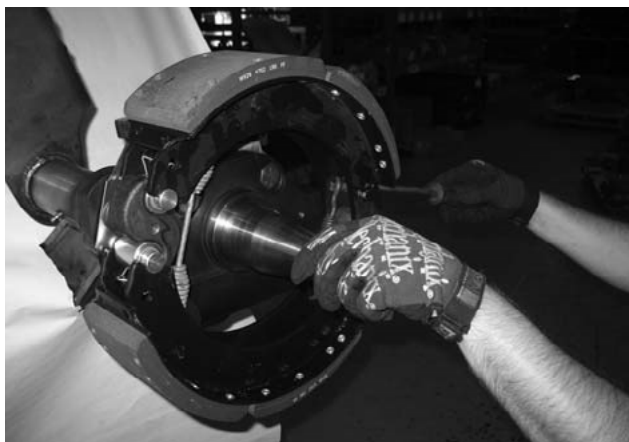
Figure 27. Removal of Outer and Inner Retaining Spring
