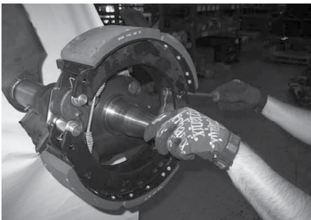
Figure 46. Removal of Outer and Inner Retaining Spring
