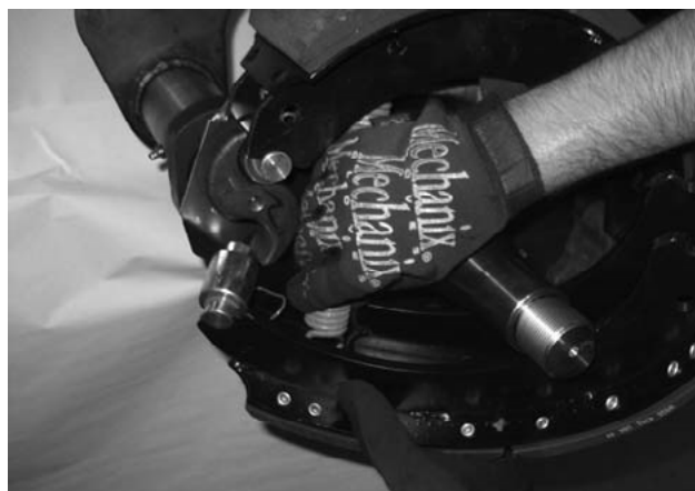
Figure 28. Removal of Return Spring
