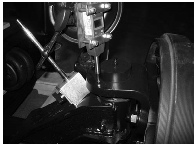
Figure 6 Vertical End Play Checking
