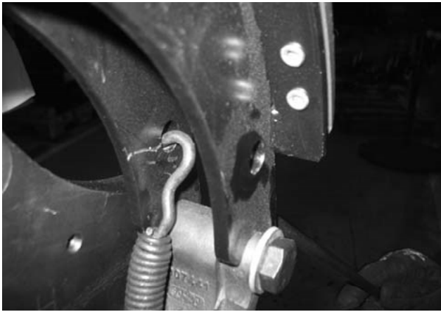
Figure 30. Spring Clipped Completely Into Mounting Hole
