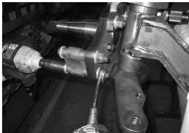
Figure 29. Removal of Brake Bolts and Anchor Pin
